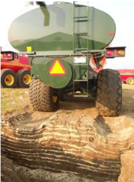
This soil pit experiment illustrates that a bias-ply tire under higher inflation pressure (right) exerts more compaction force on the soil than a radial flotation tire with lower inflation pressure (left).
