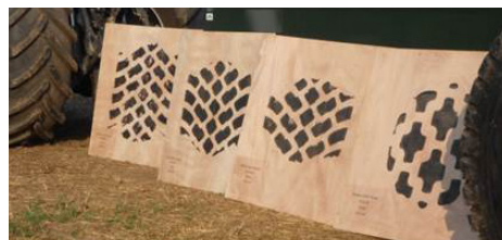
Tire design and inflation pressure have huge impacts on the footprint of a farm tire. A larger footprint distributes weight over more surface area, helping reduce soil compaction.
