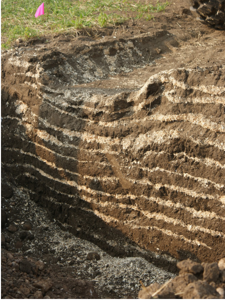
Layers of wood chips and soil reveal the compaction force of a full manure tanker on the soil. Radial flotation tires and lower inflation pressure reduce that force dramatically, minimizing compaction and keeping it in the upper few inches of the soil.
